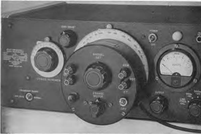
Figure 6. Close-up view of the Type 908-R X-Y Dial Drive installed on the Type 1304-B Beat-Frequency Audio Generator. This generator is ideal for audio-frequency plotting, because it covers the entire audio range in a single sweep of the dial and its output voltage is constant to \pm 0.25 db.
