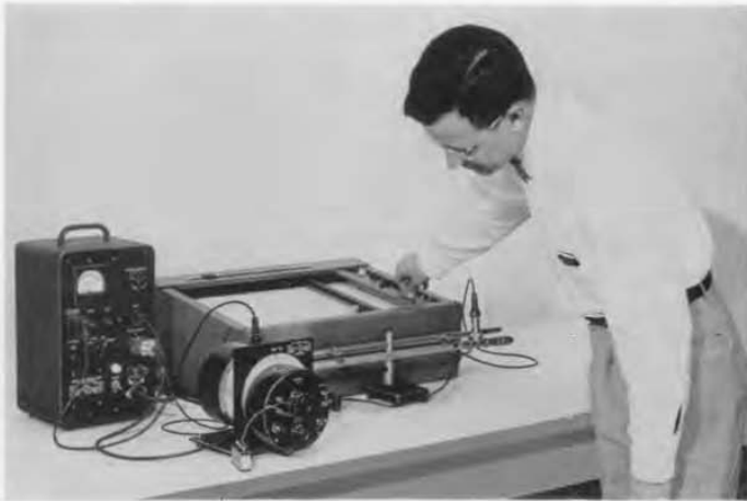
Figure 2. Assembly of equipment for plotting frequency characteristic of a Type 874-F185 Rejection Filter. The Type 1215-A Unit Oscillator is driven by the Type 908-R96 X-Y Dial Drive; oscillator amplitude is held constant by the Type 1263-A Amplitude-Regulating Power Supply. The recorder is a Variplotter, Model 1100-A, manufactured by Electronic Associates.
